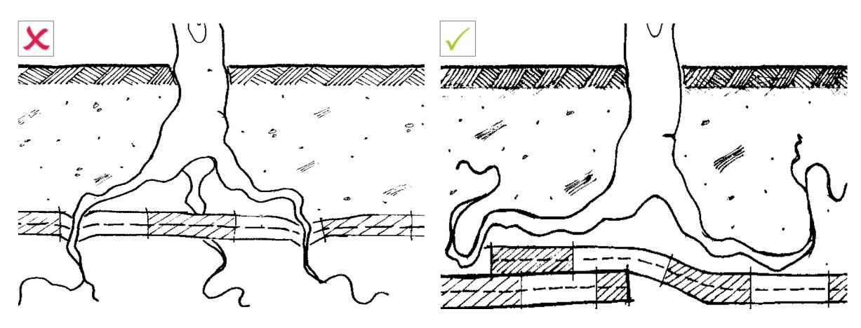
Traditional bitumen membranes are organic, so roots can grow in them, and, over the time, penetrate throughout the bitumen layer and damage the roof and waterproofing system. Bitumen membranes for green roofs contain chemical compound that does not allow roots to penetrate, at the same time it does not have a negative impact on the plant and the environment.
