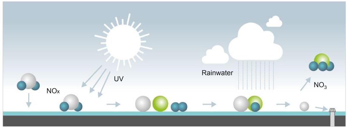
Pollution is kept on the roof surface  Pollutants and NOx are decomposed under UV rays  Harmless particles are washed away by the rainwater
