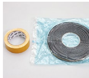
Double-sided adhesive tape — serves to seal the overlapping seams of the vapor barrier layer. Butyl-rubber tape — serves to connect the vapor barrier layer at temperatures below freezing.
