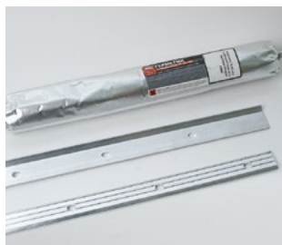
TECHNONICOL polyurethane sealant. Termination bars made from aluminium and magnesium alloy — used to fasten the edges of the waterproofing membrane to the upstand.
